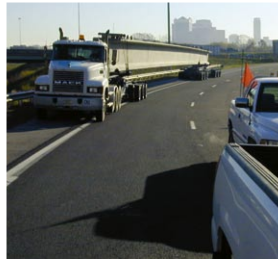
Sherman Prestressed Concrete shipped the massive girders on specially equipped 13-axle trucks. Along with the usual escort vehicles for oversized load, the Alabama State police provided additional escort for the 12-mile trip from factory to the site.
